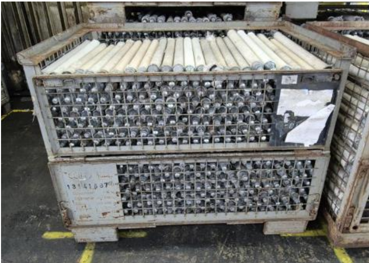
Figure 3: 700-mm stacking posts in a mesh box
